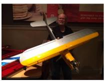
Bob Severance showed his Astro Hog Bipe that he built from a SIG kit over more than a few years. The plane is powered with a Thunder Tiger 75, 4-stroke. The pilot is a reconfigured/hand painted crash dummy. The plane is expertly covered and painted, and weighs 8 pounds. The receiver and digital servos are powered with a 6-volt NiMH battery pack.
