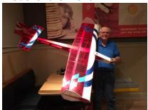
**George Wilson** showed his SLOW RIDE, advertised as "The ultimate in 3D flight". The ARF has a wing span of 63.5 inches and has a very lite wing loading. He is using AX3 for rock steady control. It's powered with a Rim Fire 28, using an 80-amp ESC and 3cell Lipo powering a 13-6.5 prop. He indicated that even though it has plenty of power to go fast, the instructions recommend keeping the speed low to avoid flutter.
